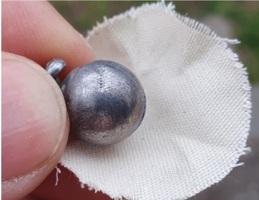
3. Imprints on a patched roundball removed from the muzzle
