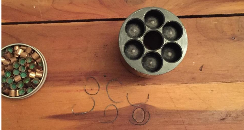
12. Loaded cylinder of a muzzle loading revolver removed from the frame. Below the sheared off lead rings are visible. (source: imgur.com)
