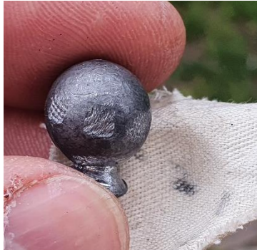
5. Marks of the rifling imprinted in the lead round ball through the patch
